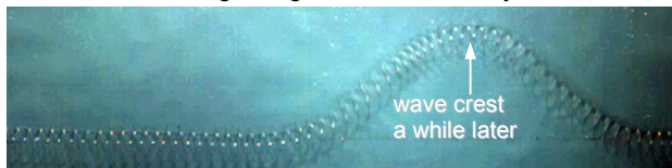
Figure 1b: A single frame showing that the transverse disturbance has moved about \frac{1}{2} meter in \frac{1}{8} th of a second.
