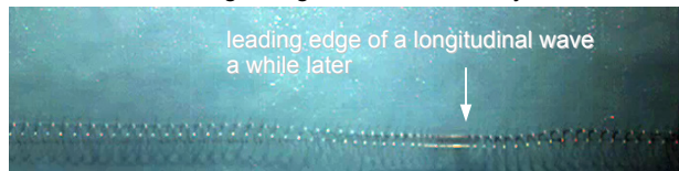
Figure 2b: A single frame showing that the longitudinal disturbance has moved about \frac{1}{2} meter in \frac{1}{8} th of a second.
